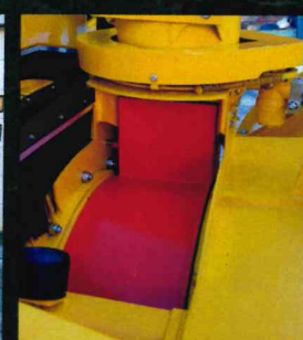
Turnable impeller housing in combination with 220° slewing ring
