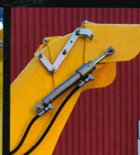
Standard chute with double flap
